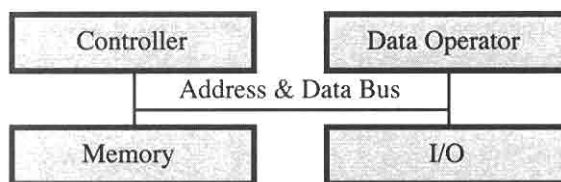
Figure 1.1. Simplified Computer Structure
